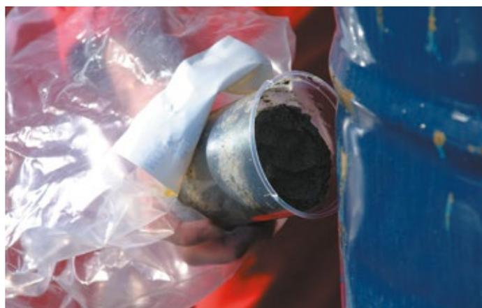
3. Push onto leak for immediate seal
