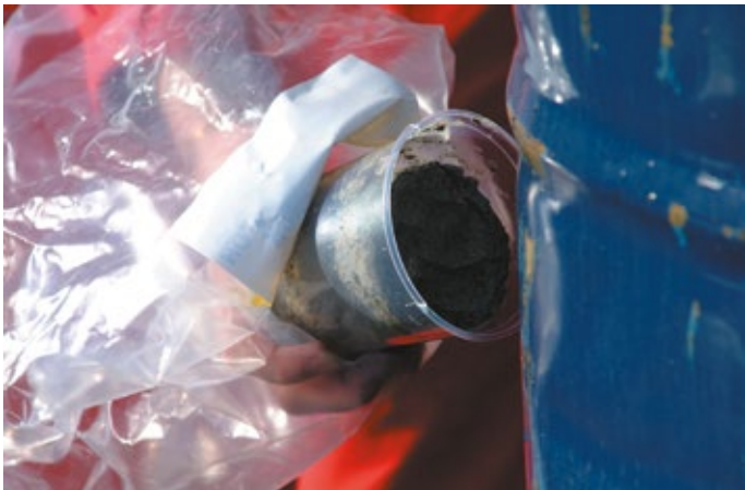
3. Push onto leak for immediate seal
